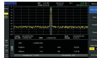
Advanced Measurement Functions - Occupied Bandwidth Measurement
